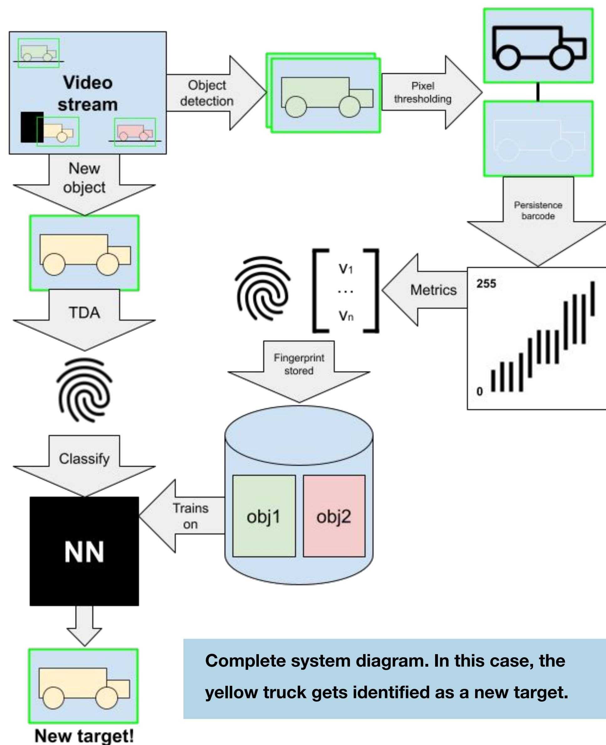
Complete system diagram. In this case, the yellow truck gets identified as a new target.
