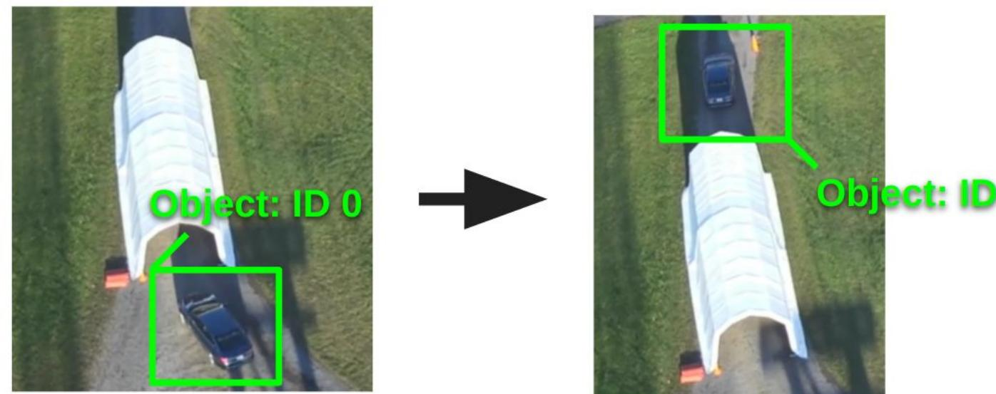
While modern convolutional neural network (CNN)-based computer vision systems are highly effective at identifying and tracking objects which are continuously in frame, they fail to persistently reidentify targets which become occluded by static objects in the environment, such as trees or buildings. TDA methodologies provide a potential solution to this problem, as a classifier can be rapidly trained on topological features of an object.
