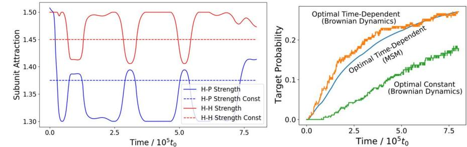
The computed optimal protocol begins with parameters that give fast but low yield assembly, then transitions to parameters that give slower, but higher yield, assembly.
