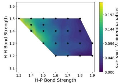
We construct local MSMs at each node in the feasible 2D parameter space (left) by sampling trajectories. Radial basis function interpolation is used to evaluate the transition probabilities away from the nodes. The interpolants can be used to build an estimate of the system transition matrix for non-sampled parameter values.
