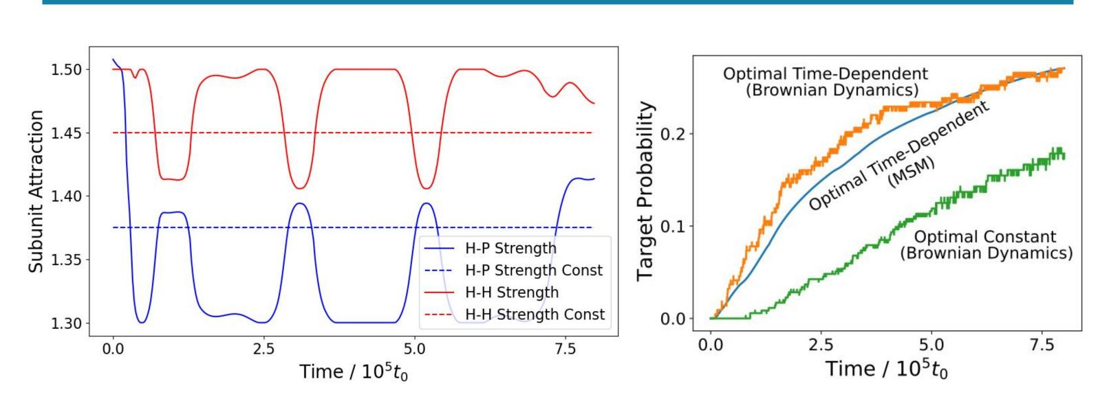
The computed optimal protocol begins with parameters that give fast but low yield assembly, then transitions to parameters that give slower, but higher yield, assembly.
