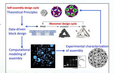
The design process consists of two nested loops of data-driven design cycles. In the monomer design cycle, colloidal monomers are built from DNA origami with sub-nm precision. In the self-assembly design cycle, the monomers join into a hierarchy of shapes.
