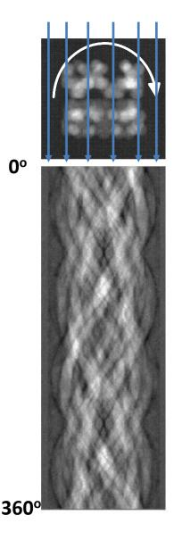
Project through the 2D image, obtaining line projection (which is the real space version of a central section of the 2D FT)
