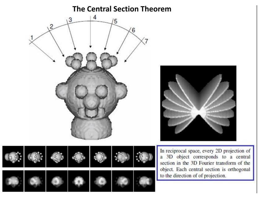
Trying to get all of the representative views of a particle is analogous to filling in the 3D fourier Transform with central sections.
