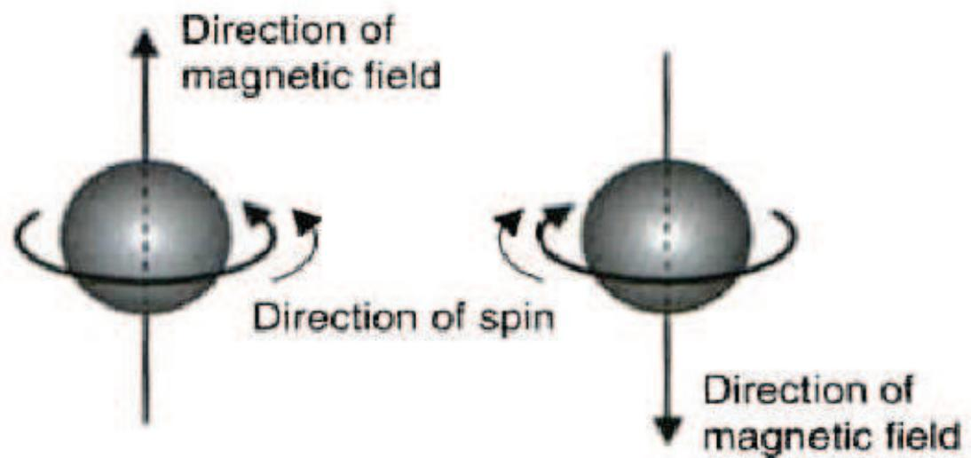
An external magnetic field is required to generate the ground and excited spin states
