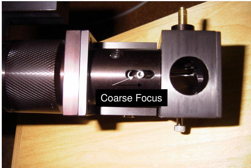
Figure 4: Coarse Focus screw on FRAP Positioning Unit
